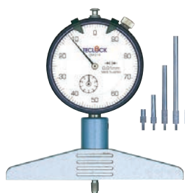
DM-214 Possible depth measurement of up to 220mm Graduation 0.01mm Measuring Range 10mm Indication Range 10mm with 5-Extension rods
